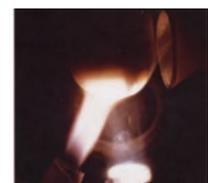
Manufacturing optical fiber preforms using the VAD method
