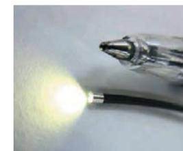
Ultra-thin endoscope using CMOS sensor
