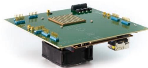
Evaluation board installed in PAAM
