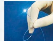
Ultra-thin fiberscope using image fibers
